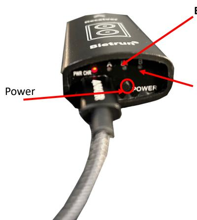
BT (Bluetooth) indicator blinking; waiting to be connected off – Bluetooth is turned off
